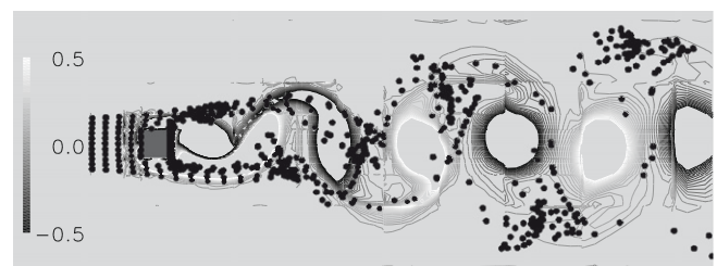
Fig. 3. Snapshots of particles with St = 5.0 periodically injected upstream and downstream of the square cylinder. The square cylinder flow at a Reynolds number, Re = 150 and free stream Mach number Ma_\infty = 0.1 sheds periodically as shown by the vorticity contours and streamlines. The particles injected downstream of the square cylinder accumulate at the square corner and shed in packages.
